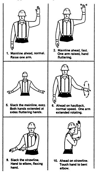
Figure 39: Standard Hand Signals
