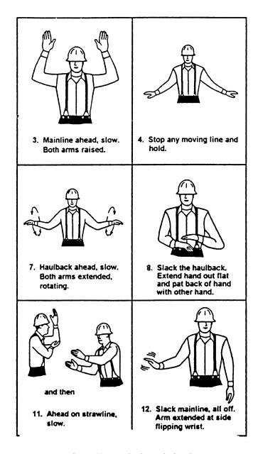
Figure 40: Standard Hand Signals
